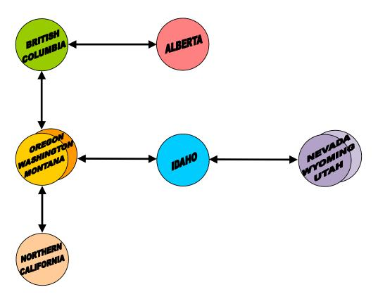
The Balancing Authorities constantly monitor critical facilities to assure availability of capacity on the transmission system for flow of contingency reserve from one zone to another. Five critical cut planes (cut planes consist of the facilities between the zones) allow for the Power Pool to enjoy maximum reliability and efficiency. If any of these cut planes become constrained, the ability to maximize reliability and efficiency is significantly reduced within the Power Pool area.
